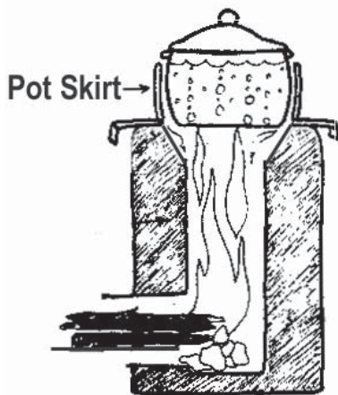
Figure 2 - Appropriate Use of Pot Skirt
