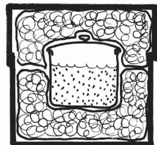
Figure 6 - Food Continues to Cook Inside the Insulated Haybox
